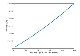
Note that the slope is always positive and becomes more positive for increasing g. The curve does not start at the origin because of startup costs, no load costs, etc.
