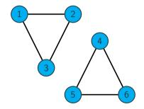
Verify that the two zero eigenvectors are (1, 1, 1, 0, 0, 0) and (0, 0, 0, 1, 1, 1) corresponding to the connected components.
